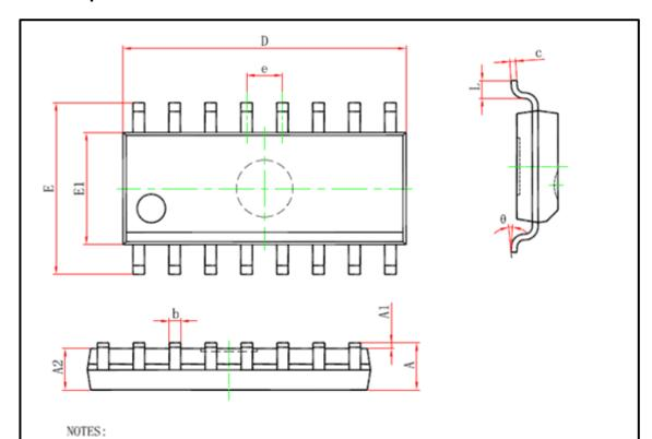
ALL DIMENSIONS MEET JEDEC STANDARD MS-012 AC DO NOT INCLUDE MOLD FLASH OR PROTRUSIONS.
